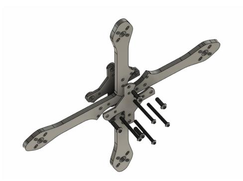
Bolt the arm assembly together with four m2.5x7mm bolts and then install the four m2x22mm stack bolts.
