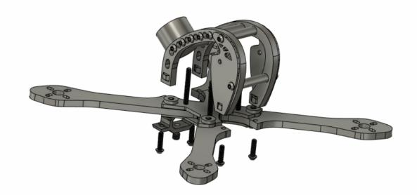
Now secure the cage to the arm assembly using two m2x8mm and two m2x10mm bolts
