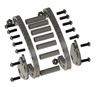
Assemble the cage assembly with 14 m2x6mm bolts, seven m2x15mm standoffs and insert four nyloc nuts into the cutouts. It is not necessary to use all of the m2 standoffs. For instance if you need to achieve a high fpv camera angle you can remove the m2 standoff above the camera.
