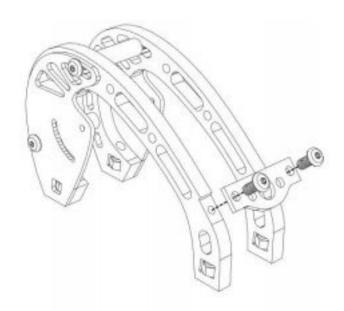
Step 5 – The top section is mounted with 2x M3x14mm bolts (back) and 2x M3x12mm bolts (front). If you don't use the XT60 connector bracket, you can use 2x M3x12mm instead of M3x14mm.
