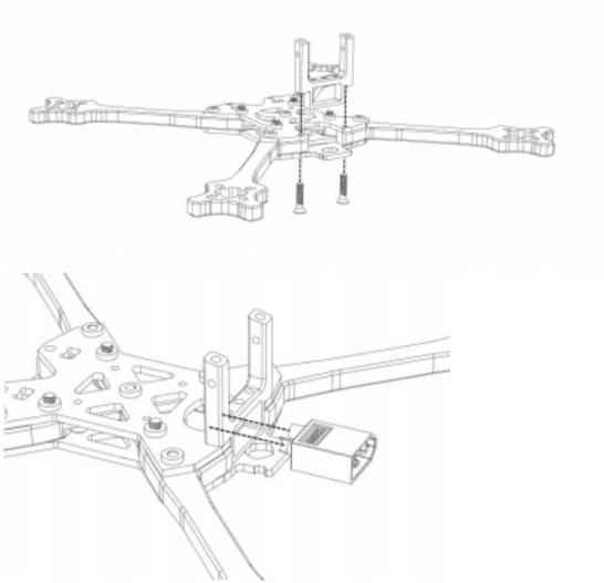
Step 4 – Next step is to assemble the aluminum front brackets and put the camera in between. Use M3x8mm button-head bolts and the supplied M3x19mm standoffs. .
