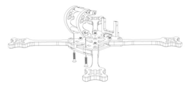
Step 6 – Lastly, put the top plate in place and use 2x M3x6mm for the front holes and 2x M3x4mm for the rear holes.
